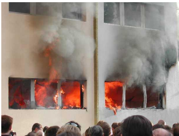
Photo: Façade fire test (after 27 minutes)
