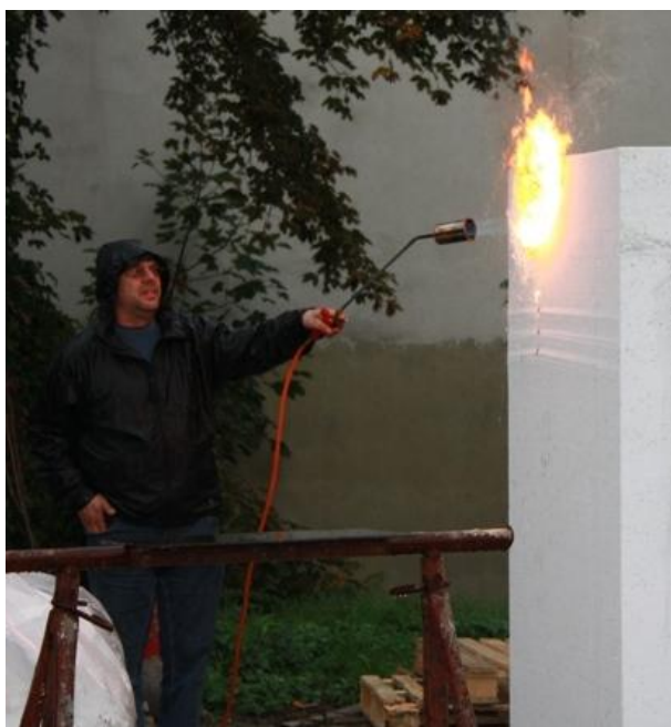
Photo: Block of constructional EPS with flame applied
