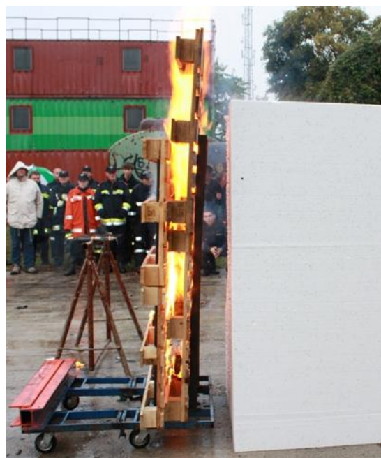
Photo: Burning wooden pallets in front of a block of constructional EPS
